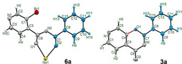
Figure 3. ORTEP diagrams of compounds 6a and 3a with thermal ellipsoids at 50% probability.
